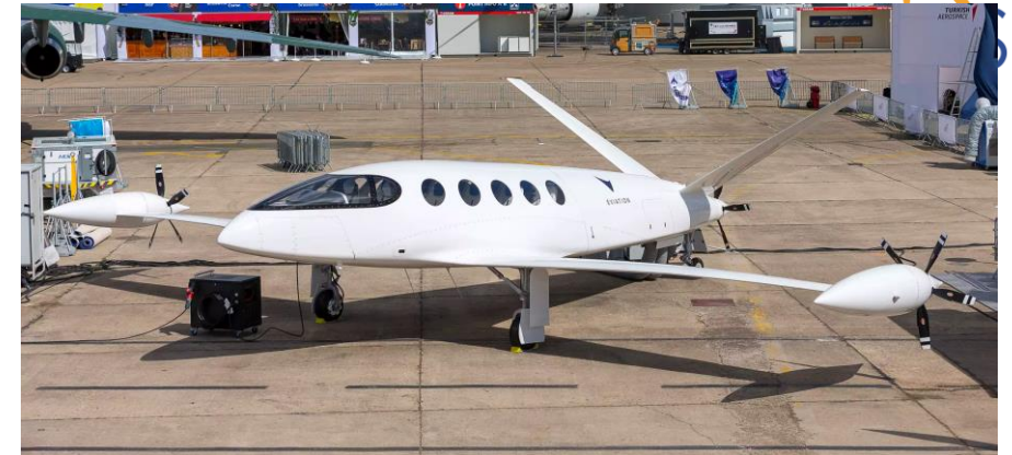
Eviation Aircraft "Alice" https://www.eviation.co/alice/ 9 passengers, 650 mile range, 275 mph, 10 000-30 000 ft, Li-ion 900kWh, propellers on tail and wingtips, $4M Planes bought by Cape Air, Barnstable MA, for short hop coastal flights
