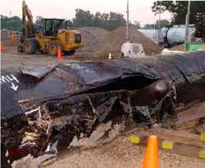
PIPELINE RUPTURE IN ENBRIDGE'S LINE 6B.
